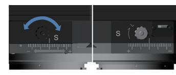
If the amount of shift is large, the lighting may be different at the top or bottom of the image, or on the left or right of the image. Therefore it is recommended to reduce the aperture value when shooting.
