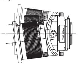
Make sure to differentiate the knob for tilting. The tilting knob is black and the locking knob is gray. Use the black knob to adjust the tilting and rotate the gray knob in the L direction to hold it in place.
